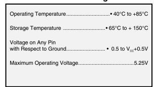
\*NOTICE: Stresses beyond those listed under "Absolute Maximum Ratings" may cause permanent damage to the device. This is a stress rating only and functional operation of the device at these or any other condition beyond those indicated in the operational sections of this specification is not implied. Exposure to absolute maximum rating conditions for extended periods of time may affect device reliability.
